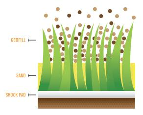
THE INFILL MATERIALS ARE PLACED IN THE TURF IN LAYERS.
